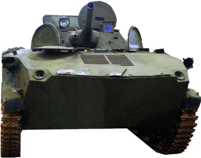
Figure 4: BMD1 at the Defence Academy Shrivenham. Note the two firing ports on the front of the hull.
