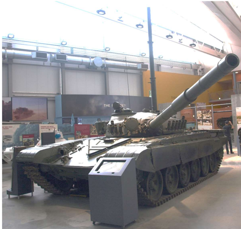
Figure 7: T72 at the Tank Museum, Bovington. Of note is the 5m high snorkel used to allow the vehicle to deep wade.
