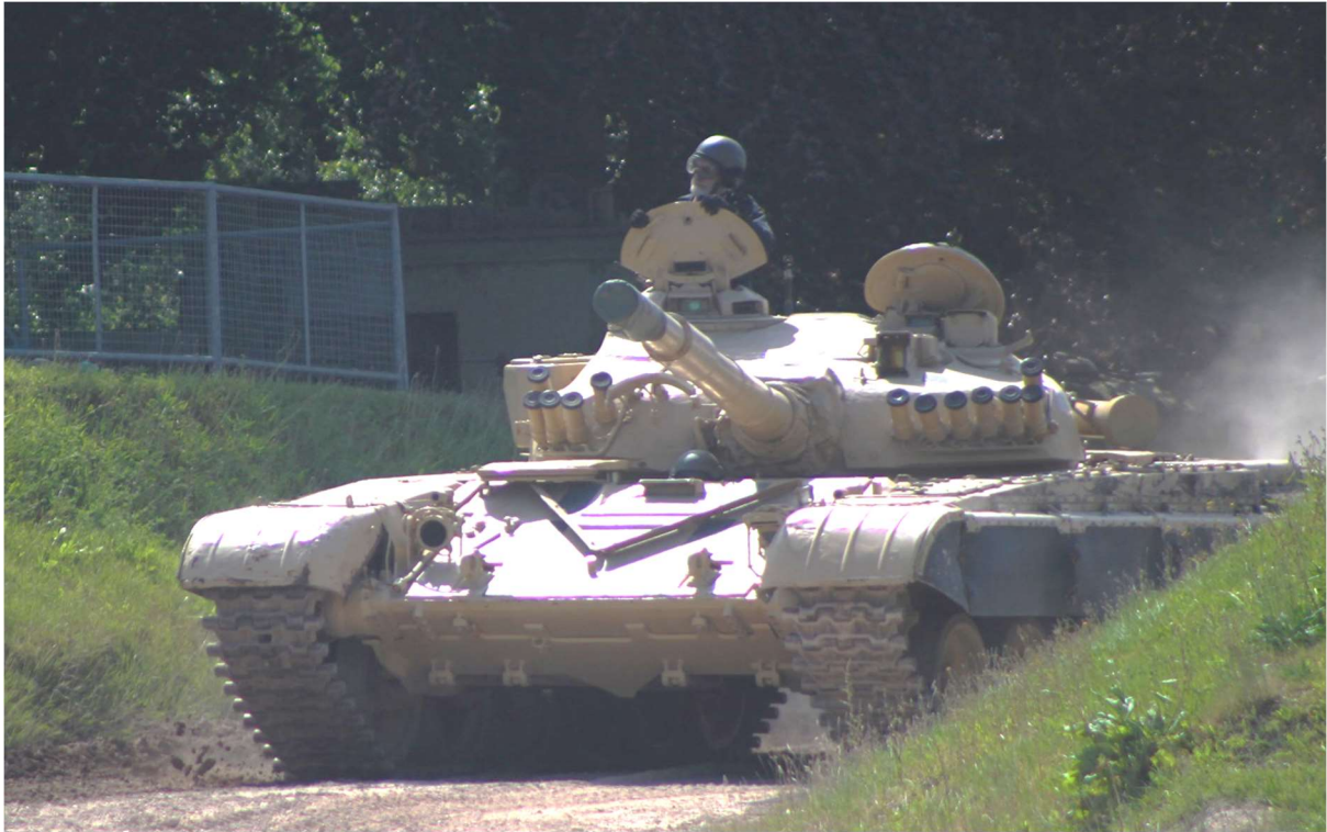
Figure 11: A T72 emerges from cover at Tankfest 2019 at the Tank Museum Bovington. Note the scraper on the lower hull that can be used in lieu of engineering vehicles to create a hull down position.
