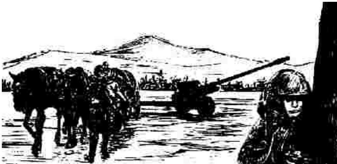
Illustration 32: Soviet Rapira-3 being towed. Note the locally manufactured limber and the horses used are cart horses resulting in the crew walking alongside or riding the limber removing the need for supporting vehicles. This solution was more common in areas where the front line was relatively static. (Pravda)
