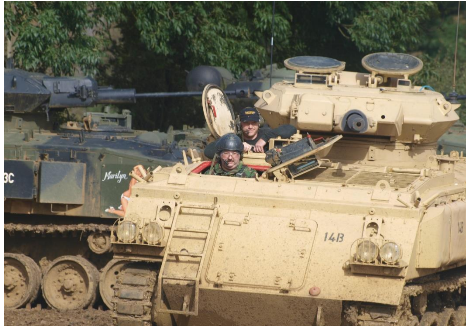
Figure 1: The author driving one of the original Berlin Brigade FV432/30s (this one was originally an ambulance version which can be identified only by examining the internal fittings). All four hatches are clearly visible in this shot. The box to the left of the 30mm Rarden cannon is the IR night vision equipment (missing its warning sign), the hole to the right is where the L7A2 GPMG would be fitted. Unusually, there is a ladder added to the hull front to aid mounting/dismounting. The vehicle was repainted in preparation to deploy to Saudi Arabia in 2007 (although in the end the unit upgraded to FV510 Warrior before deployment). Photo courtesy of Christine Appleyard
