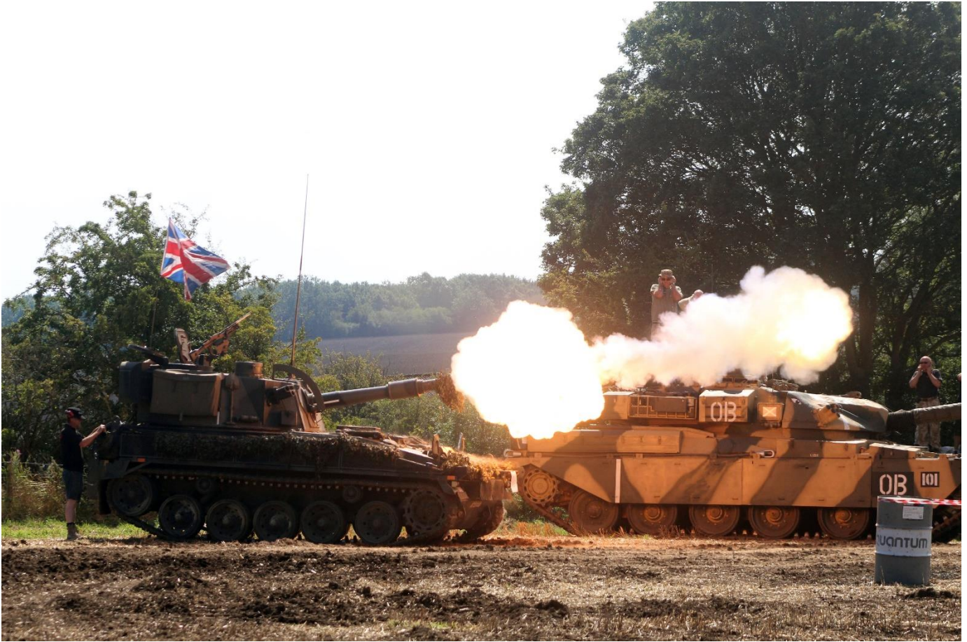
Figure 7: An Abbot 105mm gun firing at Tanks, Trucks and Firepower 2019. In the background is a Chieftain. The FV433 Abbot is a member of the FV432 series and was replaced by higher firepower 155mm armed vehicles such as the M109.
