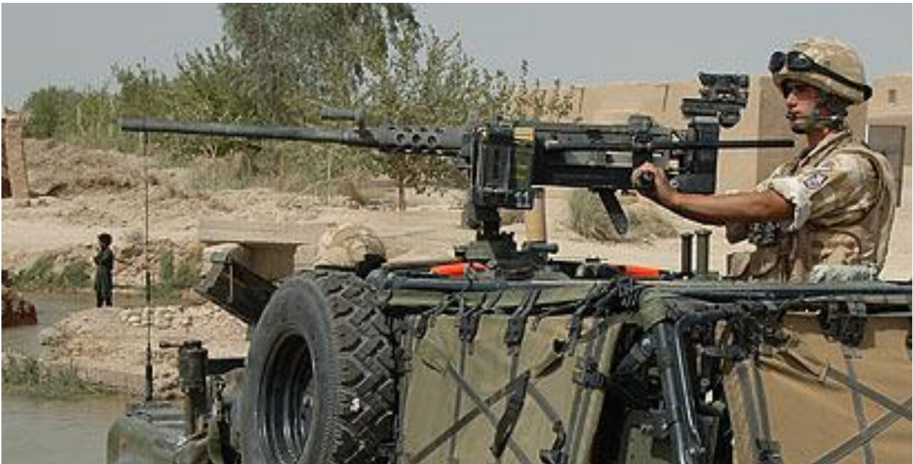
Illustration 47: 3 Para Land Rover WMIK with L111A1 MG in Iran, Spring 2000. Note the SUSAT sight, a common addition to the weapon. MoD
