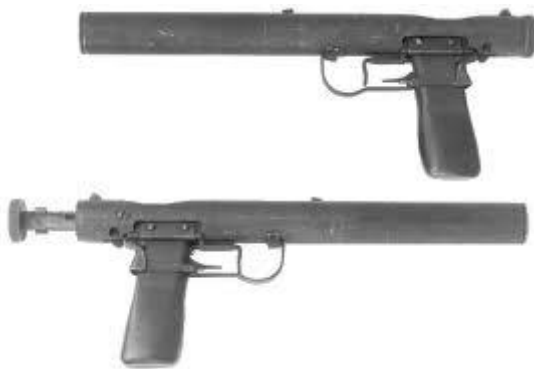
Illustration 34: Welrod Mk I showing bolt closed and open (Imperial War Museum - pre-war photo)
