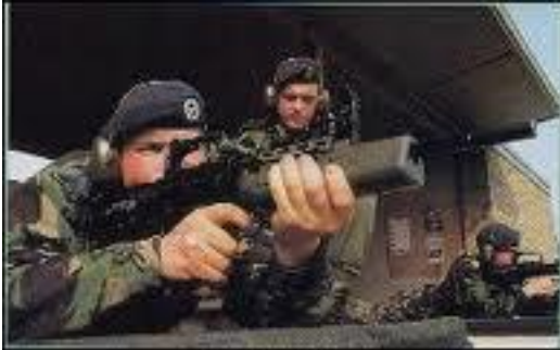
Illustration 5: L98A1 being used by Air Training Corps cadets. Note the lack of a flash eliminator, iron sights (including a post foresight) and the large cocking handle extension. MoD
